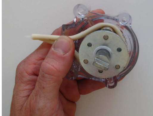
Fig. 5-20: Pump tube in the dent
