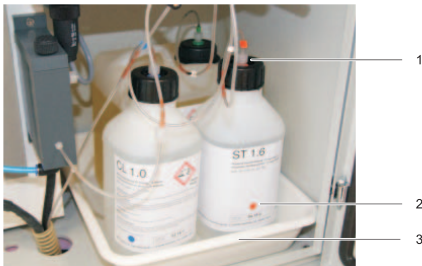
Fig. 3-19: Chemicals container (connected)
